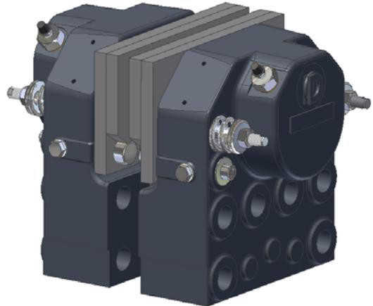
Two springs on each brake half retract the brake pads from the disc when pressure is released. Brake lining wear is automatically compensated for with increased piston stroke.
